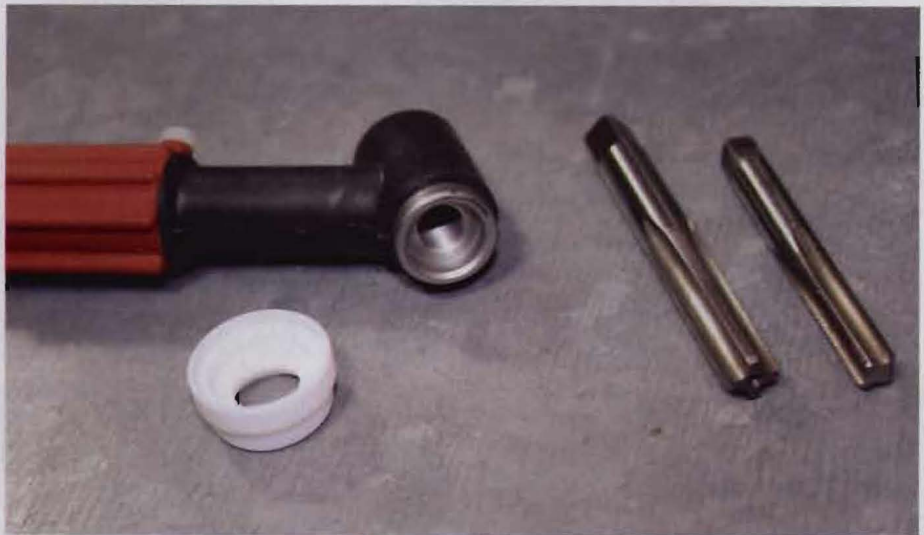
Use a tap kit periodically to chase the threads in the head to guard against thread galling.
