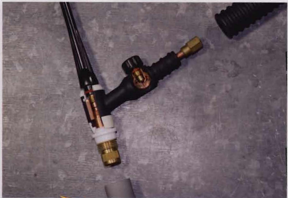
A GTAW torch is complex design and can affect weld quality negatively if poorly manufactured or maintained.
